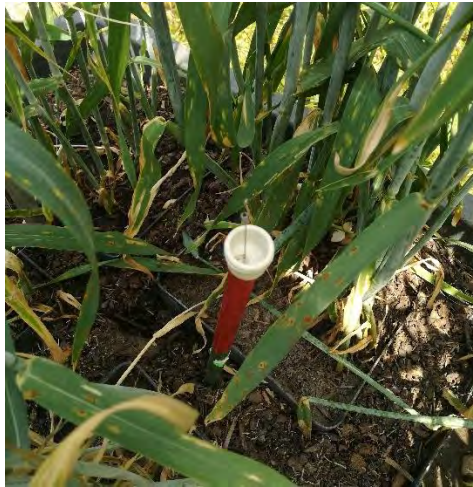
Measurement of VOCs in winter wheat via SBSE
