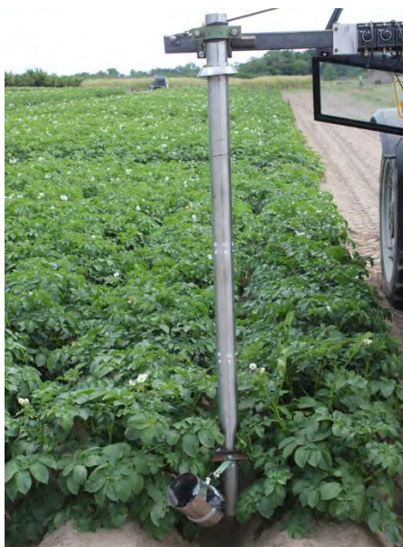
Camera-equipped vertical sensor (view skewed upwards) on the back three point linkage of the tractor for scanning the bottom of the leaves while test run in potatoes
