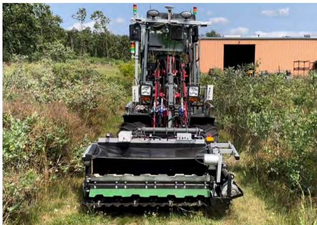
Autonomous electric tractor SunBot inside the blueberry orchard
